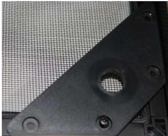
2. Using the screw driver and the included (4) screws, install all four screws. Be sure the logo on the mount is not facing you, the screws will counter sink into the provided holes. The mount must be flush on both sides.
