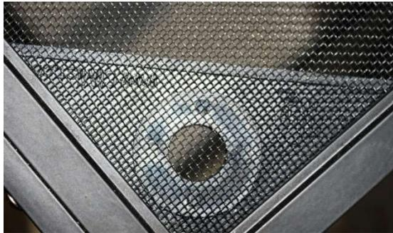
4. Place your misting assembly into the hole from inside the cage, screw hand tight the bulkhead nut. Your mount and misting assembly are now attached to the cage and you can continue installing your system.
