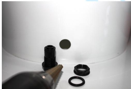
2. Take the 1/4" bulkhead with plug and gasket, unscrew and remove bulkhead nut. Insert bulkhead through the hole you made from the inside of the reservoir. The gasket should be against the inside wall of the reservoir to make a water tight seal.
